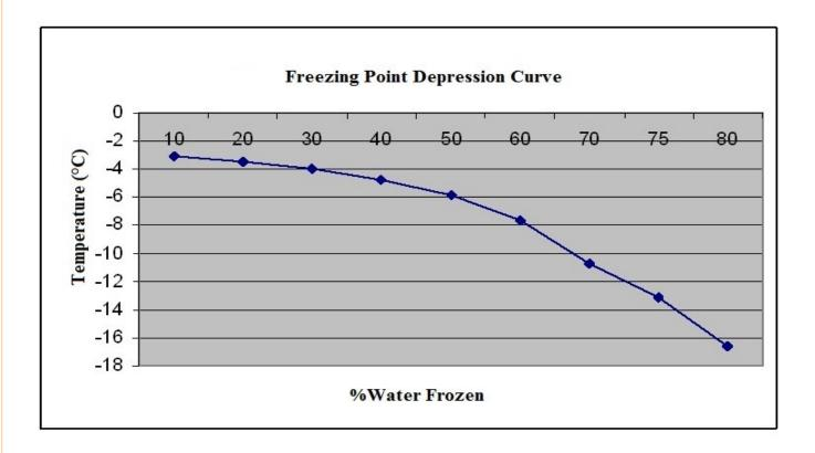
Fig. 16.3 A typical freezing point curve for ice cream mix
