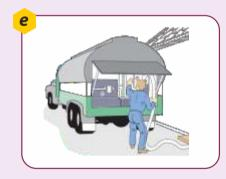
**Clean the road milk tankers** (outer barrel surface, main hole, hose pipe etc.)
