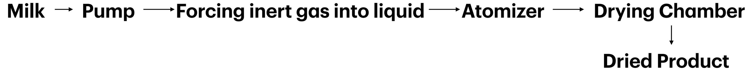
Other than drying whole milk and skim milk, this process is mainly applied to dry milk products and by-products such as butter milk, Cream (sweet and sour), whey and emulsified cheese slurry. This is done by forcing gas into the liquid product after pump but before the atomiser .
